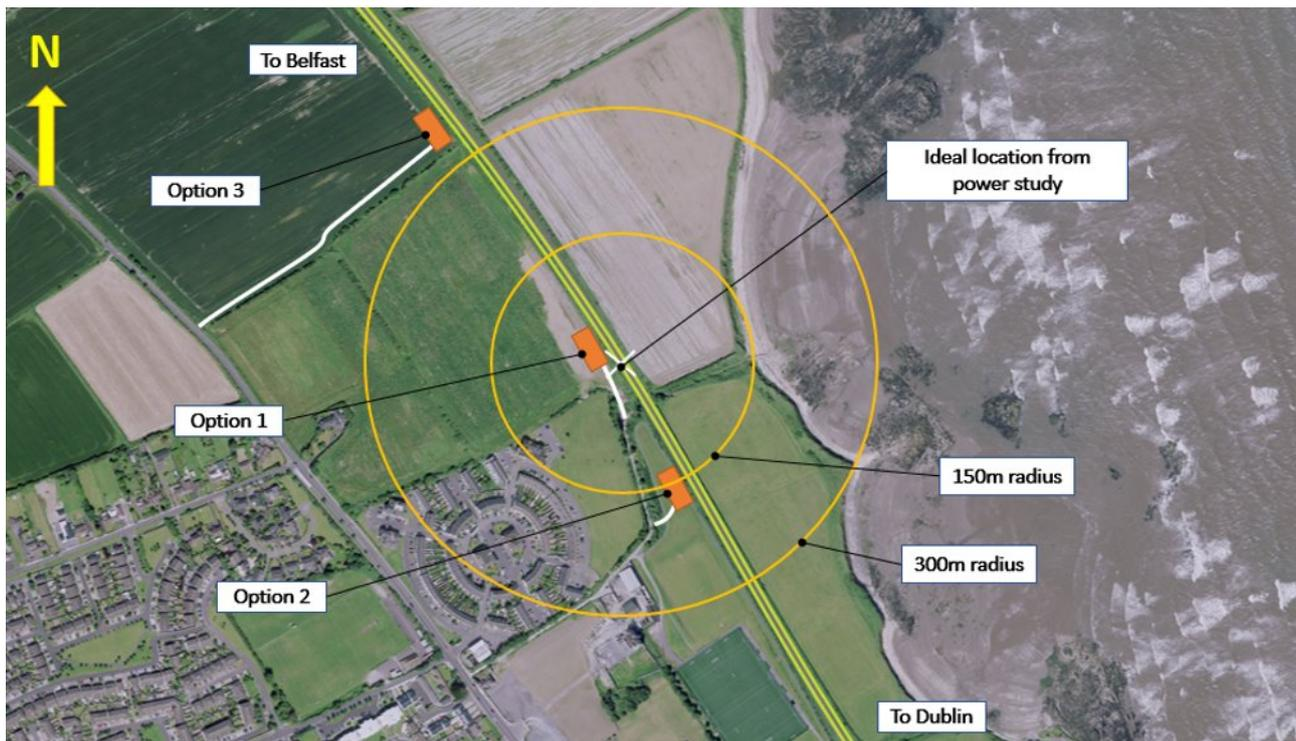
Figure 7-2: Balbriggan Substation Options
